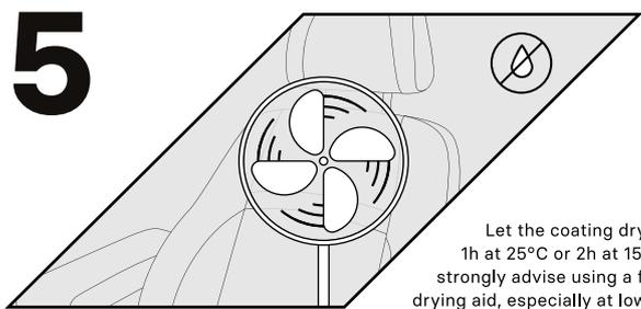
Let the coating dry for: 1h at 25°C or 2h at 15°C. We strongly advise using a fan as a drying aid, especially at lower temps.
